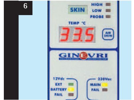
6 Skin Module. (P/N 7632). Thermoregulation of the patient skin temperature.
